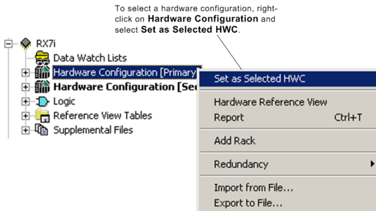
Figure 36: Select Primary Controller as Target
