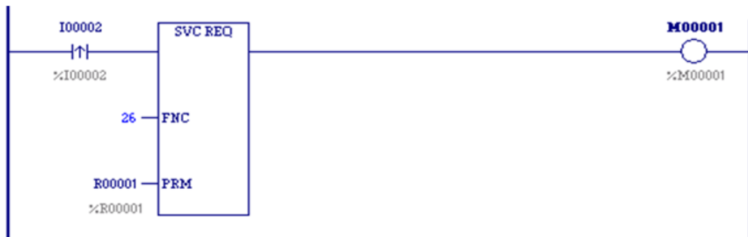
Figure 42: Ladder Logic for Role Switch (SVC_REQ 26)
