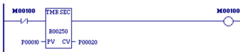
Figure 44: Ladder Logic for Synchronizing Timer
